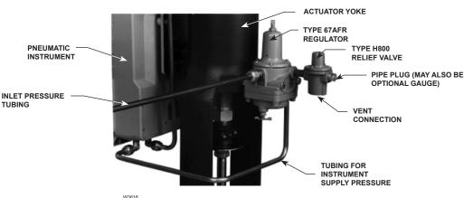
Figure 2. Typical Installation Orientations
